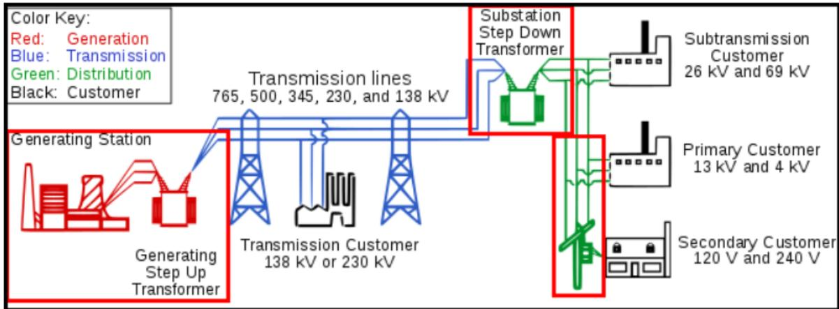
The items in the red boxes may need to be upgraded or duplicated – base load generating stations, substations, and local distribution lines including pole mounted transformers.
